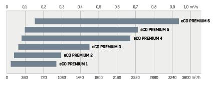
eCO PREMIUM<sup>%</sup> is available in 6 sizes providing from 0,2–0,9 m<sup>3</sup>/s of air flow. A range appropriate for a wide range of applications and building sizes.
